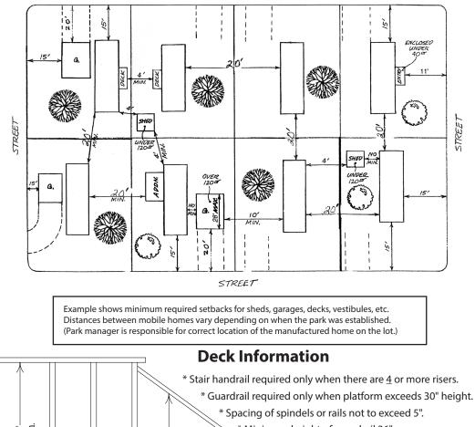
\* Minimum height of guardrail 36".
